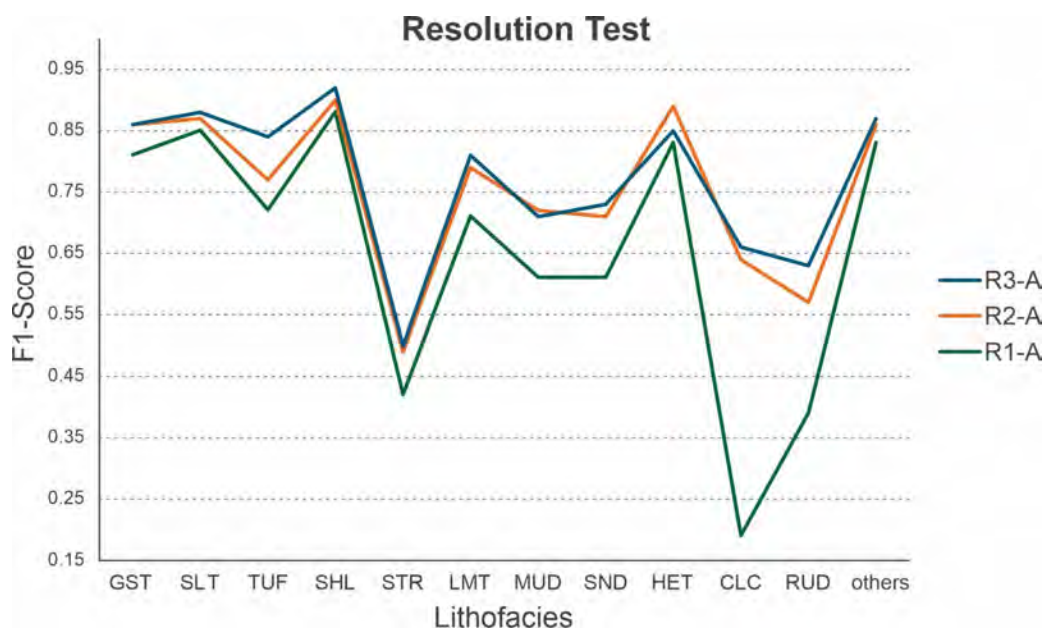
Fig. 5.7. F1-score performance for each lithofacies class across three image resolution tests on the Assado dataset: base, double, and triple resolution (R1-A, R2-A, R3-A, accuracies 78%, 83%, and 85%, respectively).
